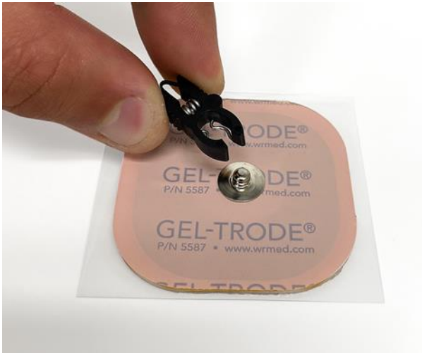
Figure 14 – Clipping Lead Wire to Gel-Trode
