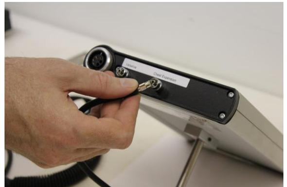
**Figure 3: Plug the Luer fitting to to the HRV Acquire main unit.**
