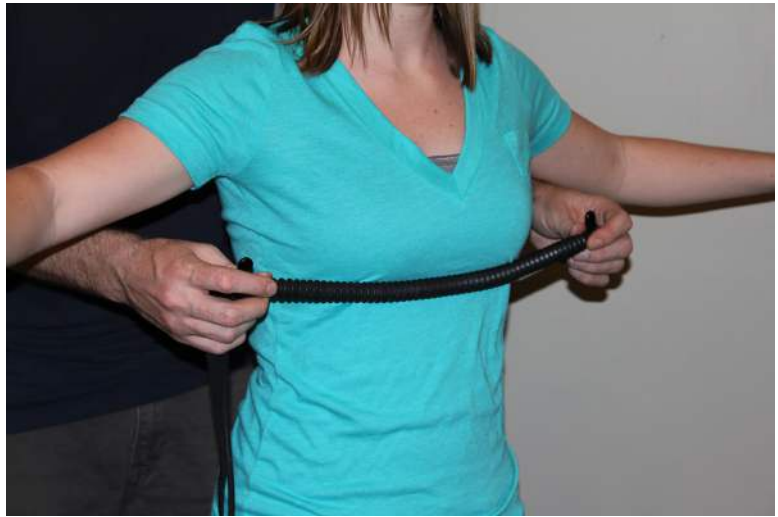
Figure 1: Attach the chest expansion bellows over the rib cage at the location of greatest expansion.
