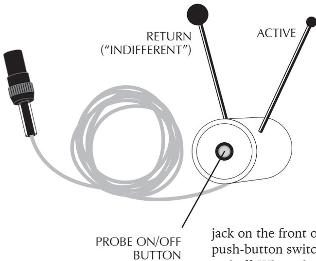
The small stainless-steel ball on the Bipolar Clinical Probe is the active electrode, and is applied to the area of the nerve trunk or branches to deliver the stimulating current. The larger ball is the return, or “indifferent,” electrode, which must also be in contact with the skin to complete the current path through the tissues. (See page 13, “Evaluating Facial Nerve Excitability,” for specific placement instructions.)
